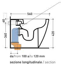
art. LK1012 (LKR90+LKR40) connessioni di scarico (in dotazione) drainage connector (included in the box)
